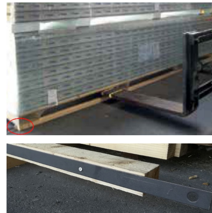
Fig. 2.7.1 Packaging for a transport in containers
