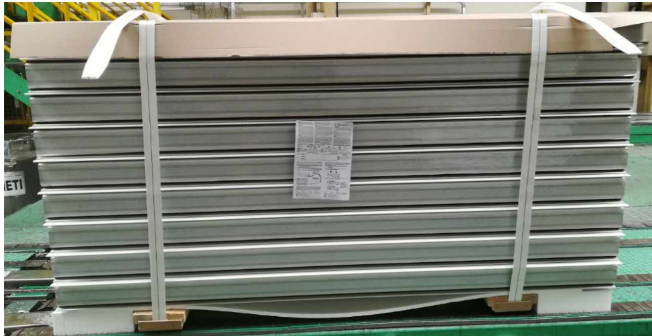
Fig. 2.6.3 Lifting band location on package
